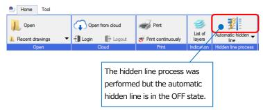
When you apply an automatic hidden line to the drawing for which hand operated hidden line was set, Rebro changes the setting details to automatic hidden line. If you want to recheck the state of hand operated hidden line, open the drawing again.
